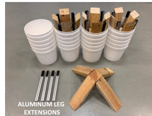
Figure 3: (LEFT) These small omni bucket stands can be stacked, stowed, and ready to lay out in minutes with their associated Launch/Land Platform and a measuring tape. (CENTER LEFT) For multiple lane transport, the stands can be stacked in fabricated caddies with the buckets stacked separately. (CENTER RIGHT) The stands can have gate hinges at the joints to stow even smaller. (RIGHT) All four hinged stands and buckets fit into two golf bags for transport. The Launch/Land Platform needs to be cut down into 12in strips with duct-taped seams acting as “accordion hinges” to fit in the golf bag along with all the buckets. The sensor panels can be cut down and taped similarly. So an entire Open Test Lane fits into two golf bags.
