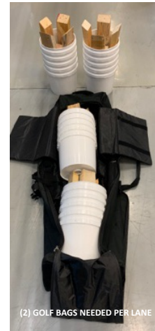
Figure 3: (LEFT) These small omni bucket stands can be stacked, stowed, and ready to lay out in minutes with their associated Launch/Land Platform and a measuring tape. (CENTER LEFT) For multiple lane transport, the stands can be stacked in fabricated caddies with the buckets stacked separately. (CENTER RIGHT) The stands can have gate hinges at the joints to stow even smaller. (RIGHT) All four hinged stands and buckets fit into two golf bags for transport. The Launch/Land Platform needs to be cut down into 12in strips with duct-taped seams acting as “accordion hinges” to fit in the golf bag along with all the buckets. The sensor panels can be cut down and taped similarly. So an entire Open Test Lane fits into two golf bags.
