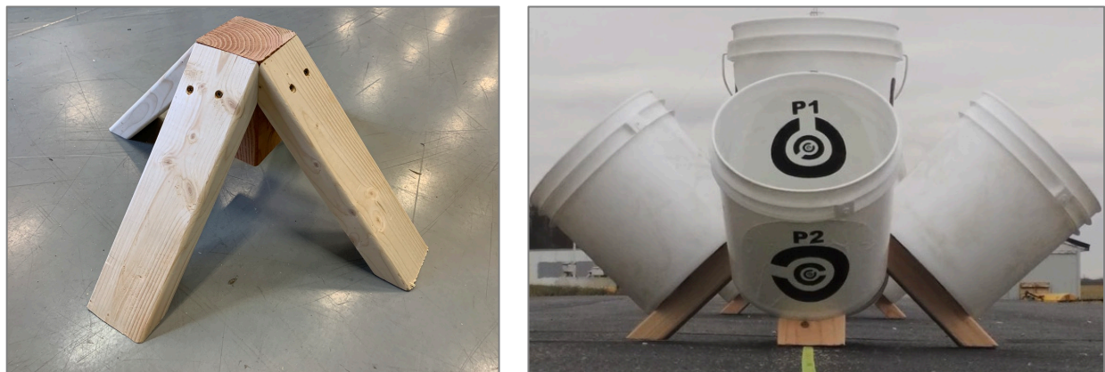
Figure 9: All four angled 5x10x30in (2x4x12in) legs with tapered ends attach aligned to the top of the center post using two 7.5cm (3in) long washer head screws. Start the screws at a 45deg angle into the legs while on the ground before attempting to affix to the center post. The top bucket mounts to the center post end grain using the same two 7.5cm (3in) long washer head screws. These need to be long to carry the weight of the entire assembled stand in the end grain. Leave the handle on the top center bucket only as a carry handle for the assembled bucket stand. The ANGLED BUCKETS SHOULD BE TOUCHING THE TOP BUCKET to support it when stacked. NOTE: Drill small drain holes in the bottom of the buckets if they are to remain outside.
