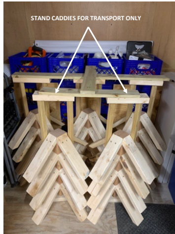
Figure 3: (LEFT) These small omni bucket stands can be stacked, stowed, and ready to lay out in minutes with their associated Launch/Land Platform and a measuring tape. (CENTER LEFT) For multiple lane transport, the stands can be stacked in fabricated caddies with the buckets stacked separately. (CENTER RIGHT) The stands can have gate hinges at the joints to stow even smaller. (RIGHT) All four hinged stands and buckets fit into two golf bags for transport. The Launch/Land Platform needs to be cut down into 12in strips with duct-taped seams acting as “accordion hinges” to fit in the golf bag along with all the buckets. The sensor panels can be cut down and taped similarly. So an entire Open Test Lane fits into two golf bags.
