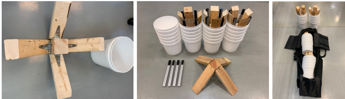
Figure 4: LEFT) The legs shown hinged underneath using 4 optional gate hinges -- $4 each. CENTER) The hinges are a bit harder to assemble, you need a bit extender, but they provide for the most compact stowing. The even fit into their associated bucket stack. RIGHT) They're probably mostly useful if you are transporting the lanes in a vehicle or as checked baggage on airlines (like anybody else would do such a thing!).
